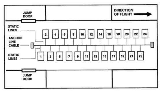
Figure 19-3. C-7A configuration for jumping from the doors.
