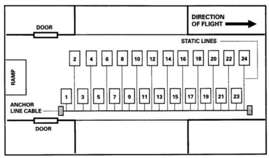
Figure 19-2. C-7A configuration for jumping from the ramp.
