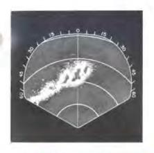
The range switch is still in the 60MI-15MRK position; however, the master switch is now in the CTR position. This display shows areas of heavy turbulence. An area of heavy rainfall is displayed at 0 degrees/35 nautical miles. Smaller areas of light rainfall are shown at 15 degrees left of the 0-degree reference and 35 degrees left of the 0-degree reference at a range of approximately 30 nautical miles.
