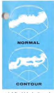
Steep gradients are displayed on the radar indicator as relatively large cores surrounded by a narrow ring of bright returns. Conversely, if cores are not displayed or if they appear as small centers surrounded by a wide ring of returns, relatively little turbulence exists. The inner and outer edges of the bright returns surrounding the black areas are two contours approximating rainfall rate.
