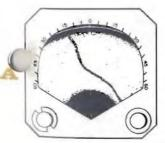
**C. GROUND-MAP INTER-PRETATION.** An aircraft flying over terrain which includes a river is shown in the accompanying illustration diagrams A, B, and C. These diagrams show the terrain as scanned by the radar beam. The aircraft is flying at an altitude of approximately 10,000 feet with an antenna tilt of 6 degrees below the horizontal plane. A segment of terrain approximately 19 miles wide is scanned by the radar system.
