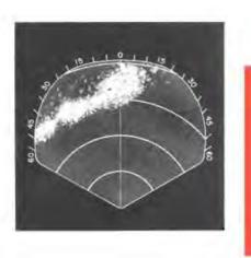
The range switch is now in the 60MI-15MRK position; the master switch is in the OPR position. The closest portion of the front is displayed approximately 30 degrees left of the 0-degree reference at the distance of approximately 40 nautical miles.
