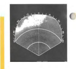
The RANGE switch is now in the 30MI-10MRK position and the master switch in the OPR position. The bright, intense echoes indicate active turbulent areas. No information is presented, however, relative to areas of rainfall and degree of turbulence.
