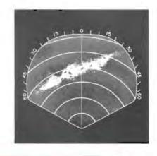
Initial detection of the weather front is made with the RANGE switch in the 150MI-25MRK position and the OFF-STBY-OPR-CTR switch (master switch) in the CTR position.
