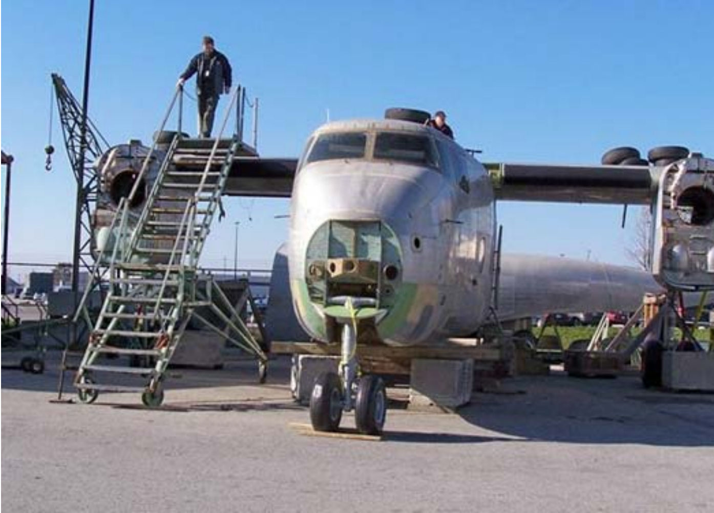
Back out into the light of day, the main wing section is mated to the fuselage main section. Photo via www.buffalo461.ca
