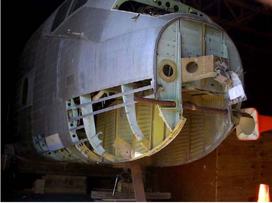
The wheel well section (taken from the junkyard Buffalo found in Newmarket, Ontario) has been joined to the main fuselage prior to final attachment and skinning. Photo via www.buffalo461.ca
