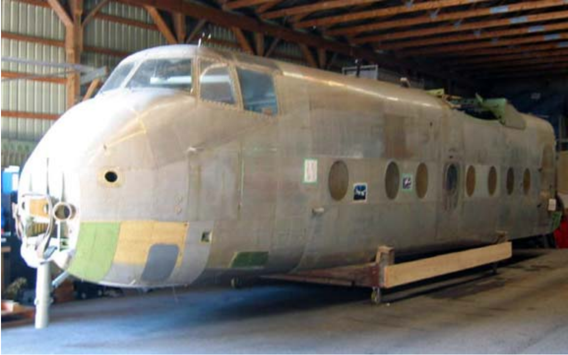
A photo taken shortly after work was completed on the nose section and wheel well sub-project. The well is installed and the outer skin panels now block out the ravages of Canadian winters. The nose gear oleo is seen in the extended position. Photo via www.buffalo461.ca
