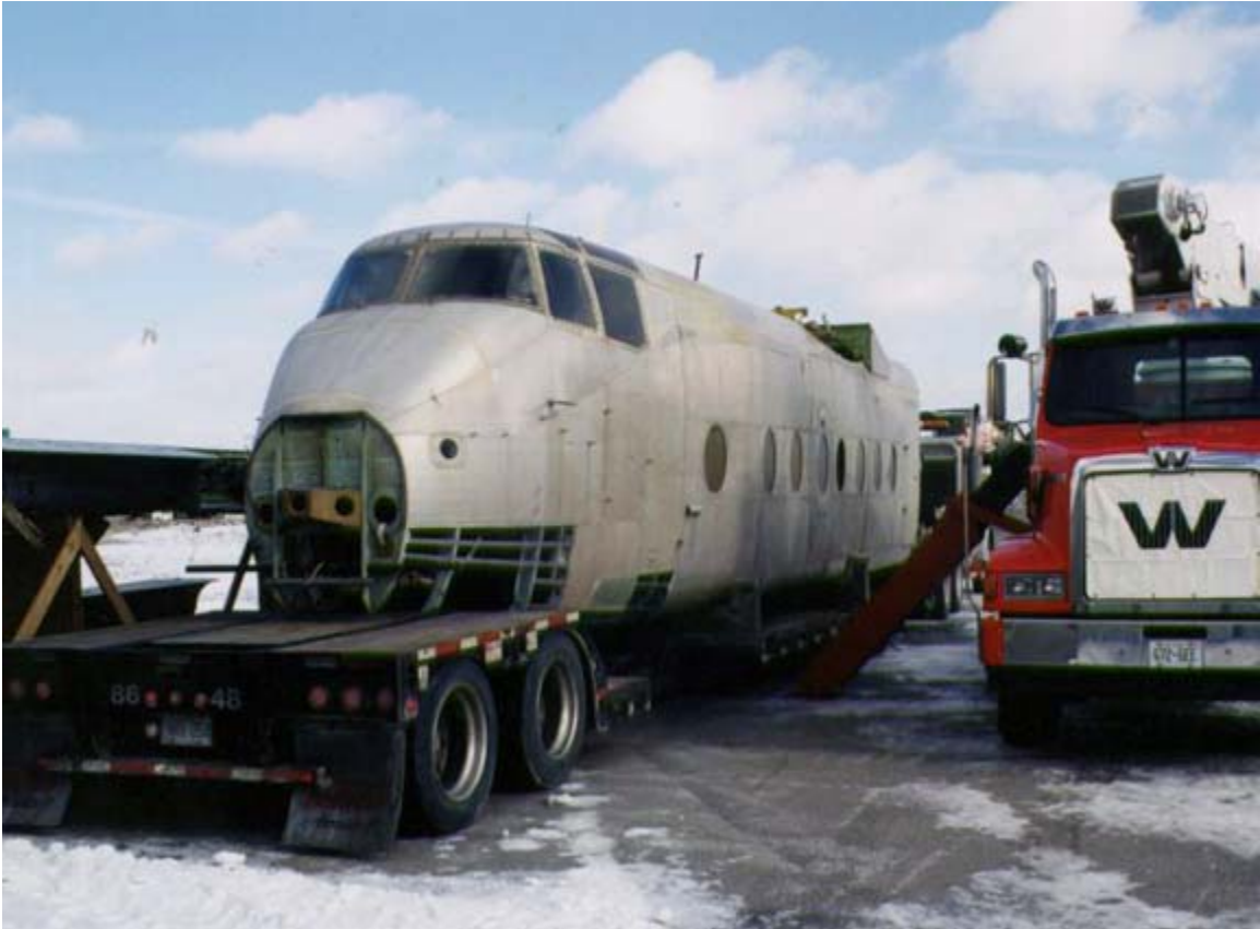
The fuselage sits on a flatbed trailer outside the Canadian Warplane Heritage Museum, while a crane donated by Aurora Crane sidles up next to it to lift the big pieces to the ground. Here we can see the completely exposed nose section where the wheel well is supposed to be. Photo via www.buffalo461.ca
